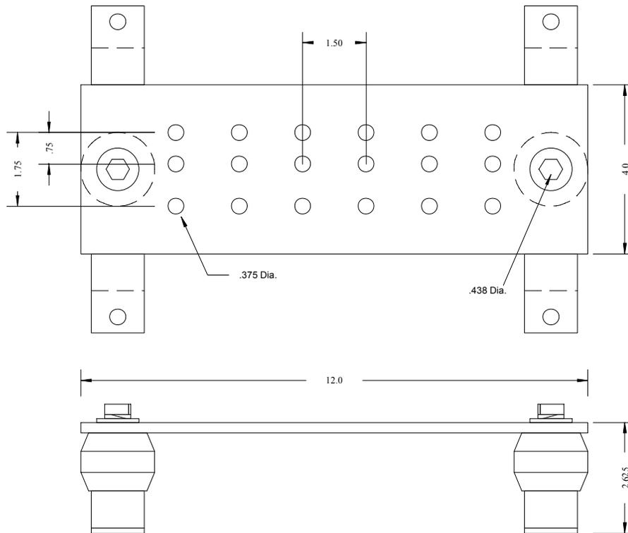
Standard busbar assemblies are insulated and specifically designed for commercial applications. The silver washed 110 alloy copper ground bars are 1/4" thick and stand off 2.625" from the wall or backboard.
